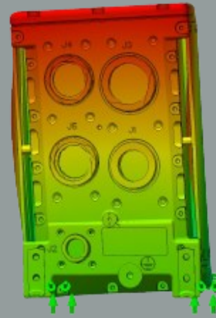
A deformed results plot showing accelerated loading of the unit in the XY (traverse) plane.
