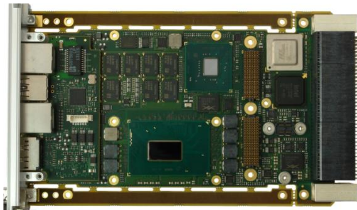
FIGURE 3 - TOP VIEW OF A 3U VPX SBC WITH COFFEE LAKE POSITIONED OFFSET FROM THE CENTRE [2]
