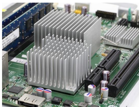
FIGURE 1 - A TYPICAL "STICK-ON" HEATSINK FOR ELECTRONICS APPLICATIONS
